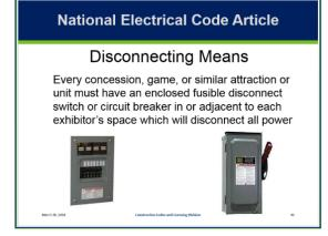
installed outdoors must be rainproof, unless otherwise protected from the weather
